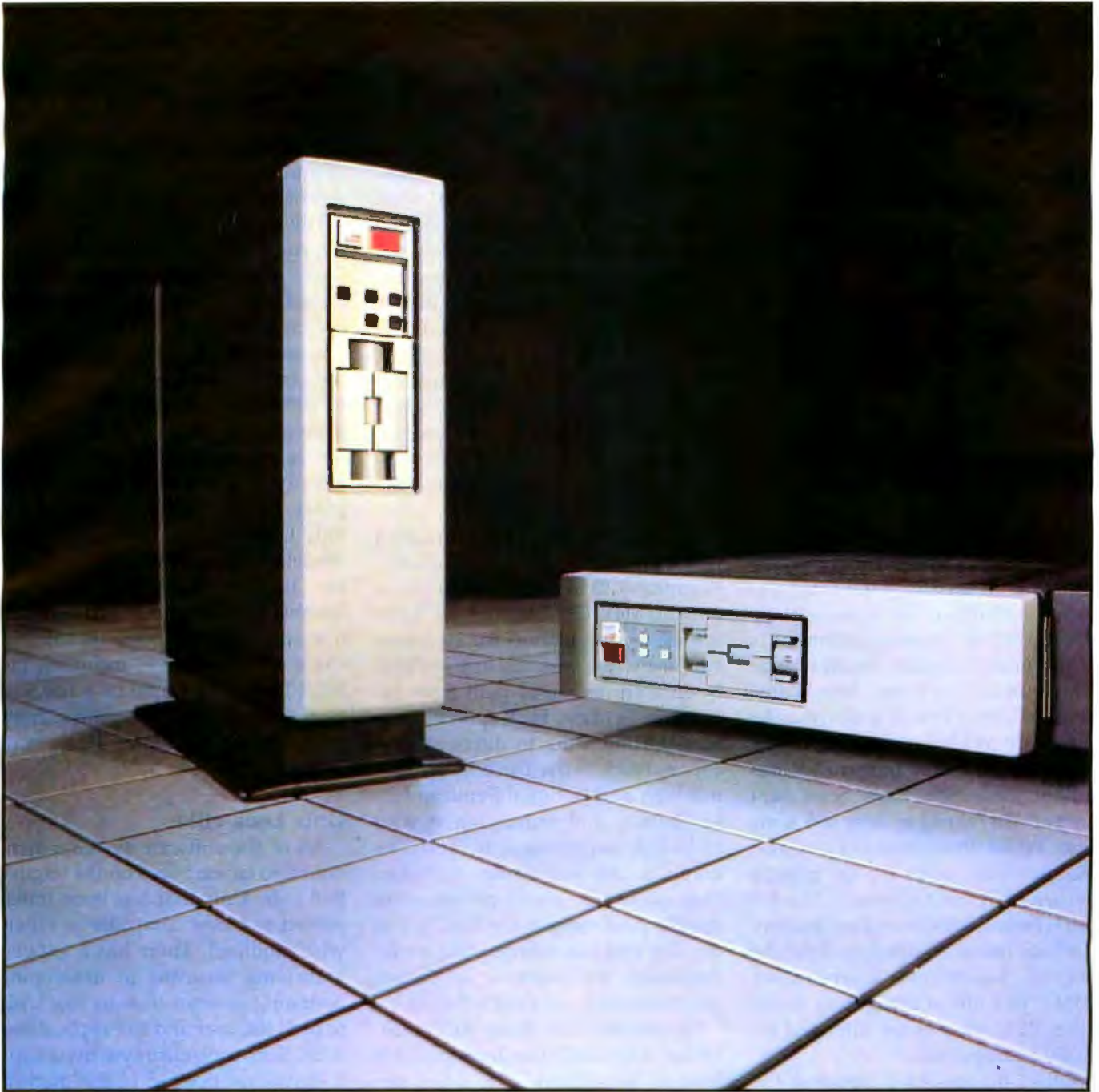
Photo 1: Digital Equipment Corporation's Micro/PDP-11 is a microcomputer version of the original PDP-11 that Unix was developed on. The system has a 10-megabyte hard disk (with floppy disks for backup) and 256K bytes of memory.
