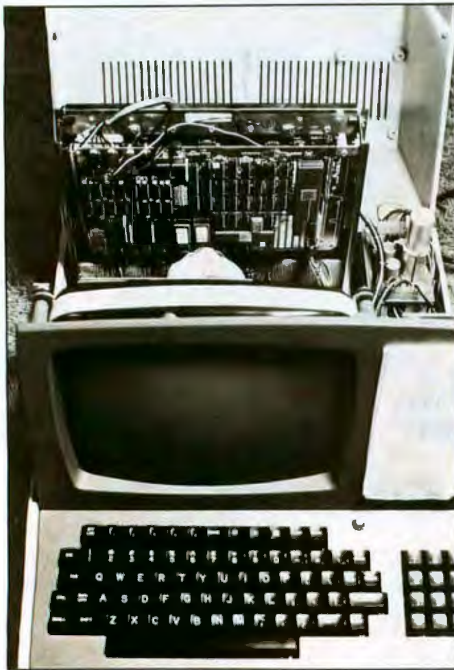
Photo 4: The ECB fits neatly into a Heathkit H-19 terminal. Regulated power is obtained from the H-19 through the wires in the upper left. The serial output of the terminal goes directly to the ECB, and the host port of the ECB is wired to the serial output port of the H-19. Separate holes punched in the rear chassis are for the cassette and disk I/O connectors.
