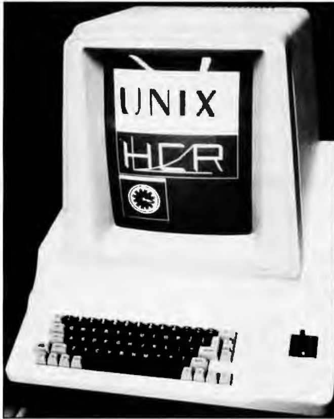
Photo 1: The NS16000 workstation, which includes memory-management and floating-point capabilities. This workstation was used to port a demand-paging virtual-memory implementation of Unix to the NS16032 processor.
