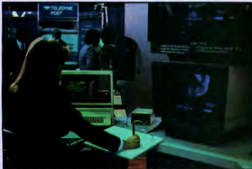
A complete graphics system that includes an Apple IIe (background left) and a Jupiter 7 (foreground right). Commands are entered with a Summagraphics bit-pad pointer.
