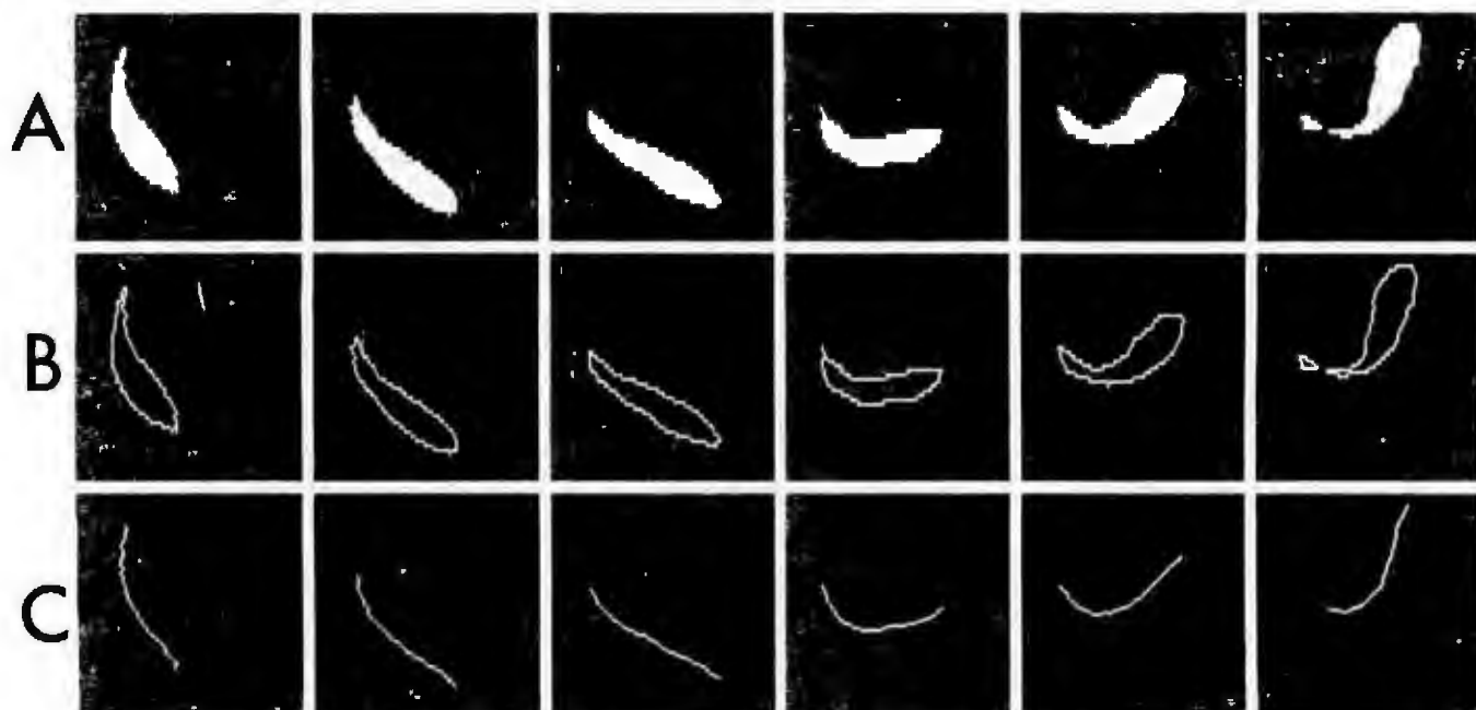
Figure 4: An example of image analysis based on a digital image generated by the Microneye. Shown are sequential frames, "filmed" from beneath a glass aquarium, of a goldfish executing a turn. Using binary image information supplied by the Microneye camera and image-analysis programs (designed by the author and not supplied with the camera), it is possible to determine mechanical properties (such as angular velocity and displacement speed) of the fish's turn. Time between each frame is 370 milliseconds. A shows the fish silhouette (the original camera image); B, the computer-generated outline; and C, the computer-generated midline.
