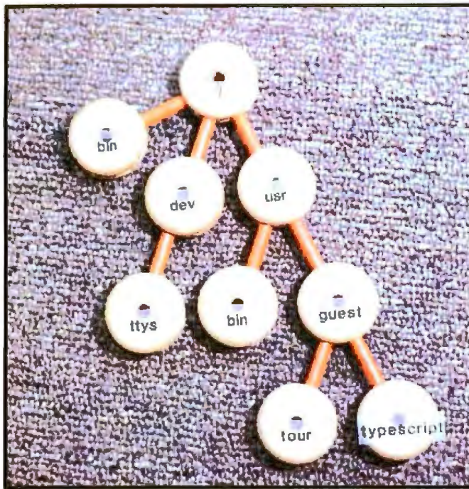
Figure 1: The relationship of directories and files in the Unix hierarchical file system. (Photo by James Joyce.)
