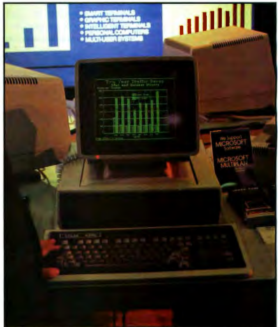
Photo 3: Visual Technology's first move from terminals to computers. This version of the 1050, with software, two drives, CP/M 3.0, and manuals, lists for $2695. True dot graphics are displayed with text. (Photo by the author.)
