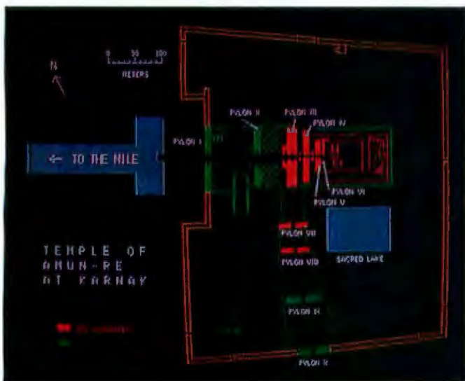
Photo 3: Examples of color graphics on the APC. Although each pixel may be only one of eight colors, different colored pixels that are close to each other appear as new hues or shades.
