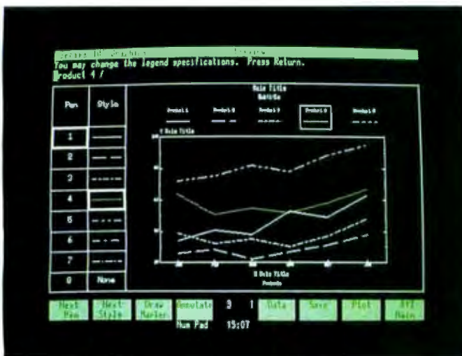
Photo 23: Series 100 graphics from HP use touch to select pen color, style, and the functions you see on softkeys.
