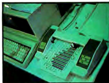
Photo 5: The Enter Computer Sweet-P plotter fits into a briefcase and is relatively light. The pen moves in one direction only; the paper moves in the opposite direction. Enter has made plots "up to 10 feet long" on the Sweet-P using this feature. (Photo by the author.)
