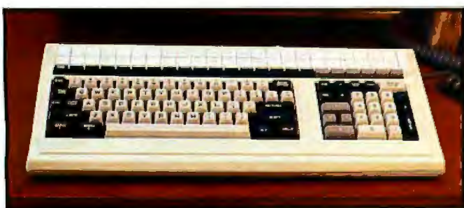
Photo 4: The APC keyboard. Twenty-two programmable function keys are above the regular keys. At the top of the keyboard is an overlay strip that can be used to indicate the programmed functions of the special keys. Notice that the left Shift key is upside down (see text).
