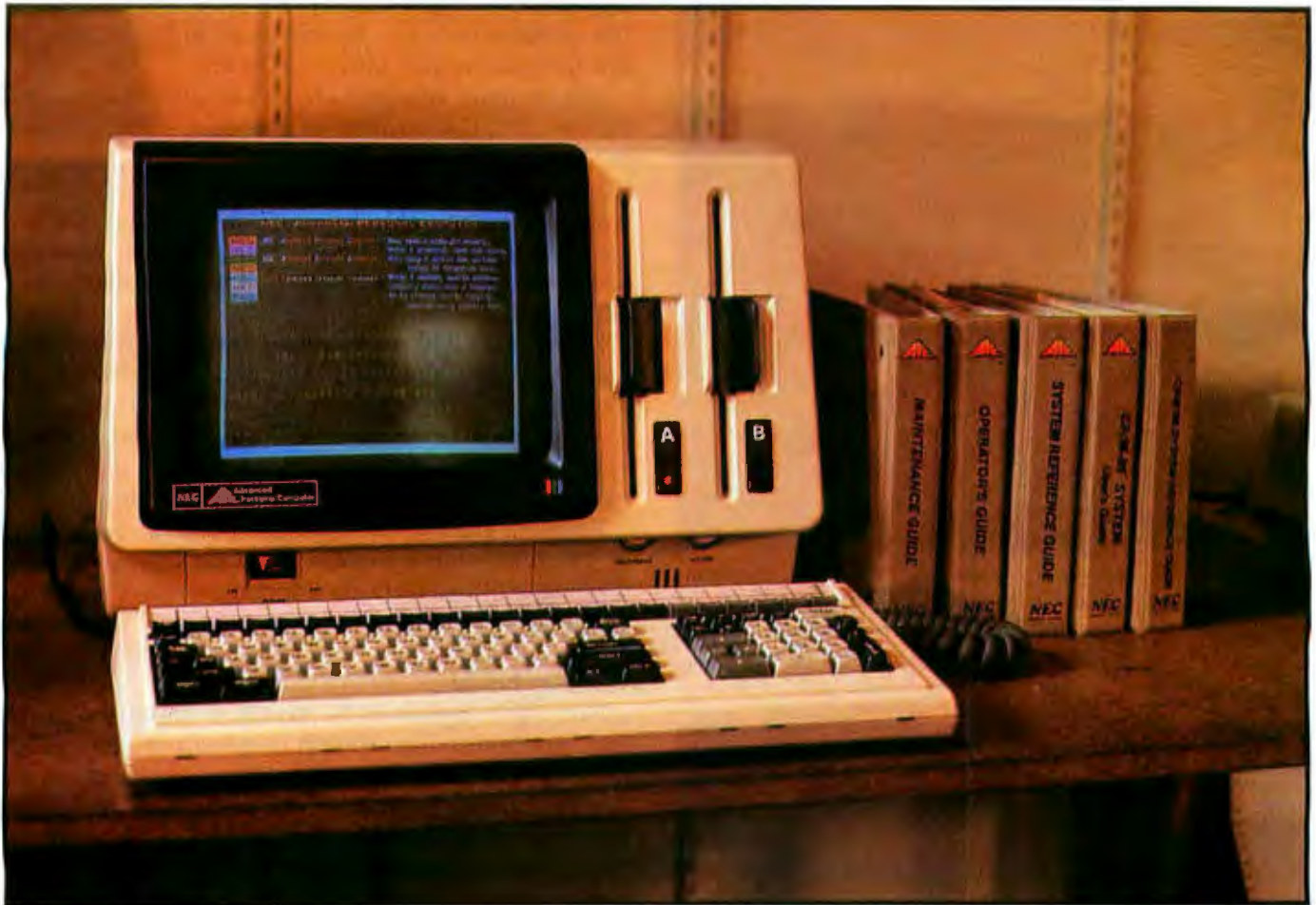
Photo 1: The NEC APC (color model), with five volumes of documentation. The main power switch is under the display. The brightness and volume controls are under the disk drives. Note the main power cord, which attaches to the front of the system.
