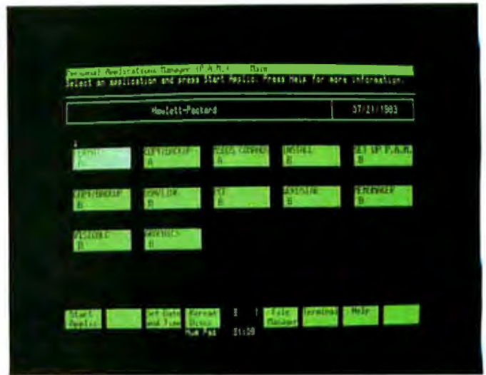
Photo 9: HP's operating system shell. Touch an application name to select it, then touch "Start Applic." to run it.
