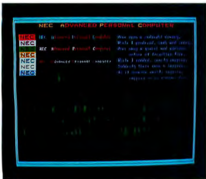
Photo 2: The APC display, showing normal ASCII characters, special characters, and user-defined characters. Eight colors are available (in normal and reverse video), plus underline, overline, vertical line, and blink.
