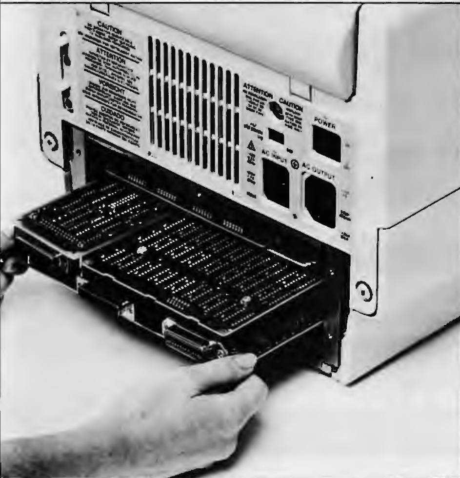
Photo 3: The motherboard holds a 256K-byte memory board on the left. The video-controller board is directly above the motherboard.
